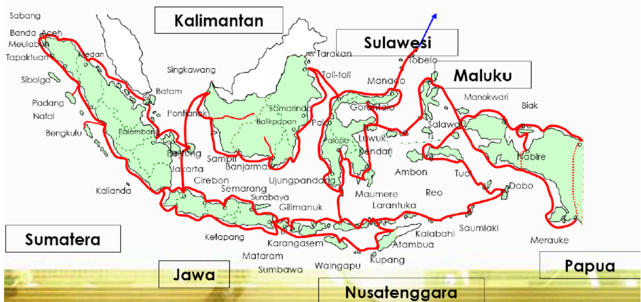
Figure 3.8 Indonesia's Submarine Cable System
